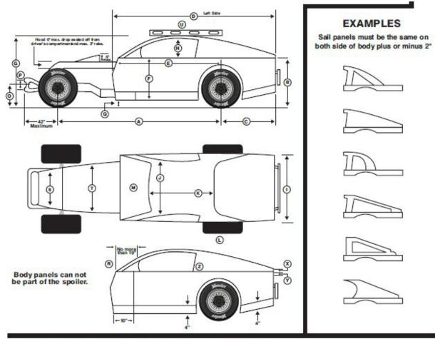
Rear bumper must be capped, with no sharp edges, and bent forward on the ends at a 90° degree angle.
