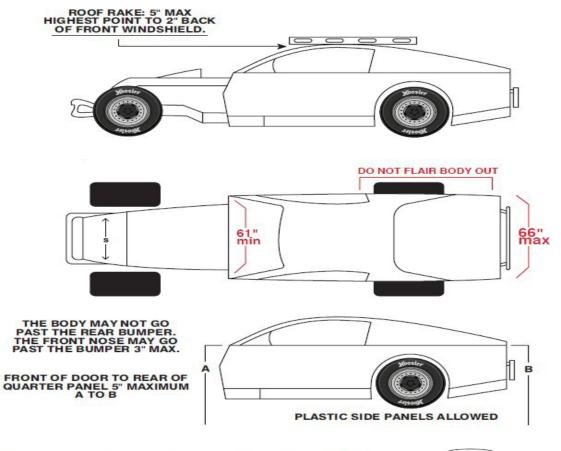
Rear quarter panel cannot be over 2" different left to right in total height. No flat or concaved roofs. Sail panels must be the same on both sides of the body and in the same location. (Plus or minus 2")
