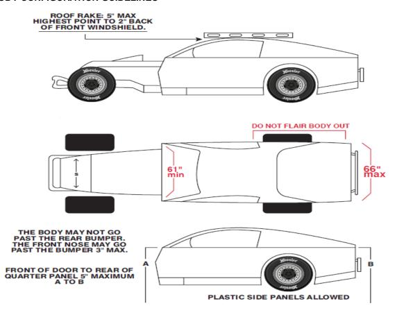
Rear quarter panel cannot be over 2" different left to right in total height. No flat or concaved roofs. Sail panels must be the same on both sides of the body and in the same location. (Plus or minus 2")
