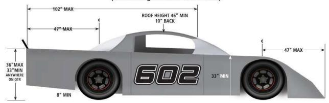
REAR DECK AND QUARTER PANEL AREA MUST BE A STRAIGHT LINE TO REAR AND TOP TO BOTTOM FROM TIRE CENTER LINE TO 47" REARWARD AND ACROSS.
